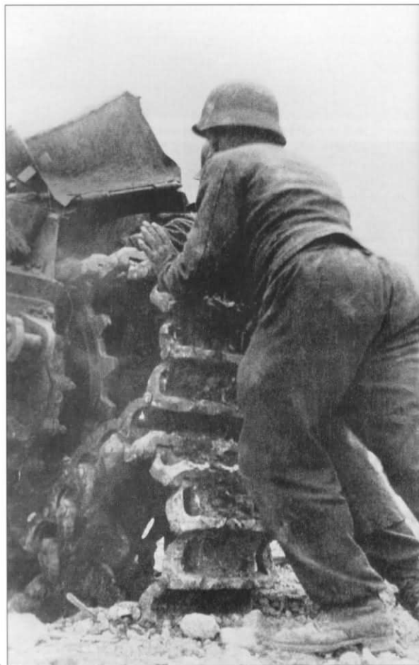
The crew of a Pz.Kpfw.IV struggles to repair a damaged track. This was a difficult job at the best of times and in action, was much more difficult and dangerous. Often, minor damage such as this resulted in the complete loss of the vehicle if repairs were impossible to carry out because of combat conditions.
