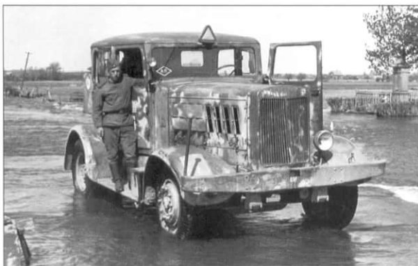
A Soviet soldier poses on this nicely camouflaged Hanomag SS100N German Army tractor which has been abandoned on a flooded road near Berlin in May 1945. Besides the original camouflage, there are a number of markings painted on various parts of the vehicle. One, on the front mudguard, has been painted over and there is one, obscured behind the soldier's leg, painted on the door. A white circle with a number in it, is painted on the rear of the body, visible over the soldier's right shoulder and a white outline diamond with the letters 'An' is painted on the windscreen.
