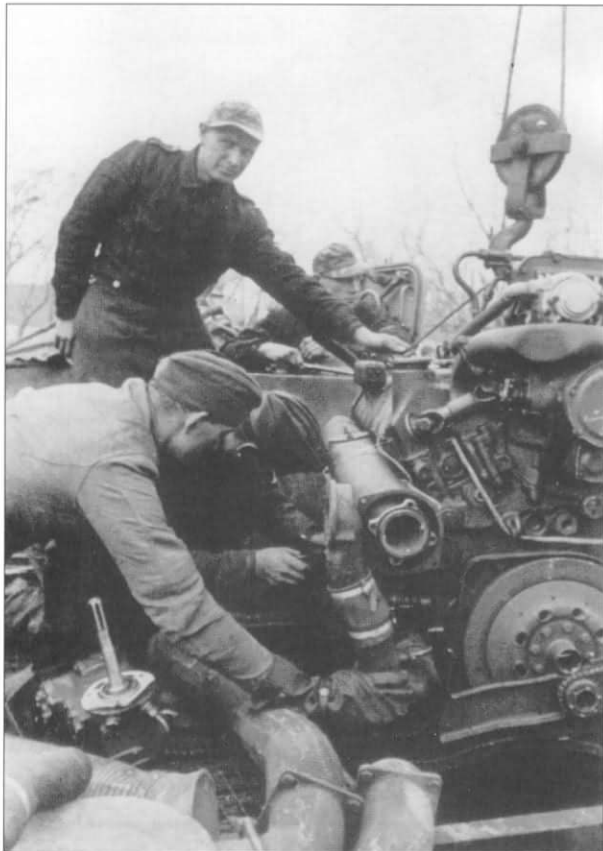
Mechanics work to replace the Maybach HL230 P45 V12 engine in a Tiger I. The 700 HP motor consumed almost 3 liters of fuel for each kilometer on the road and 5 liters over normal off-road terrain making it one of the less economical vehicles to run in the Panzerwaffe.
