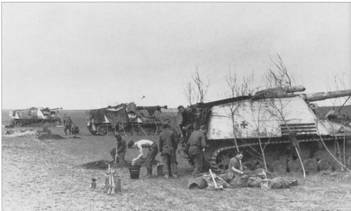
A battery of 'Hummel' self-propelled guns sit in position somewhere in Romania in early May 1944. An attempt has been made to camouflage the vehicles with branches so their winter camouflage schemes will not be so noticeable on the spring landscape. The paint was usually thinned with water which made it easy to wash off when it was no longer necessary.
