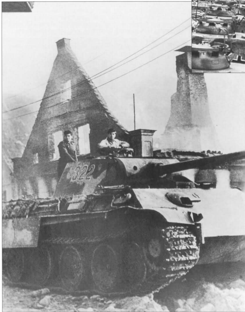
A Pz.Kpfw.V Panther Ausf.G passes through the ruins of an East Prussian city in autumn 1944. There is no zimmerit on this vehicle, indicating it was manufactured after the beginning of September 1944. It is also likely painted in red oxide primer with camouflage patches of green and dark sand that were now ordered to be applied at the assembly plants. The tactical number '322' is red with a white outline.
