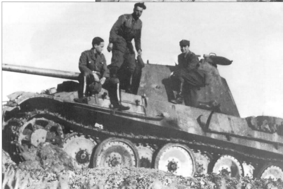
A late Pz.Kpfw.V Panther Ausf.G knocked out by the Polish Army in southern Germany during the last days of the war in May 1945. The anti-tank round penetrated the side of the hull just above the bottom of the sponson, blowing off the gun cleaning rod tube and part of the mudguard. Note that this Panther has foliage loops welded to the turret that were ordered to be installed starting in March 1945. Unusually, it still has the anti-aircraft MG rail welded to the cupola that was ordered dropped in January. The raised fan cover for the crew compartment heater can also be seen.
