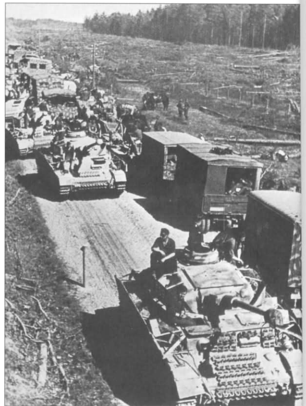
A column of Pz.Kpfw.V Panther and transport vehicles of all types on the retreat somewhere on the Eastern Front, summer 1944. The closest one is a Ausf.A and is fitted with the twin cooling pipes on the left side exhaust that were introduced in January 1944. Mud thrown up on the rear of the stowage bin has almost obscured the Balkenkreuz painted there.
