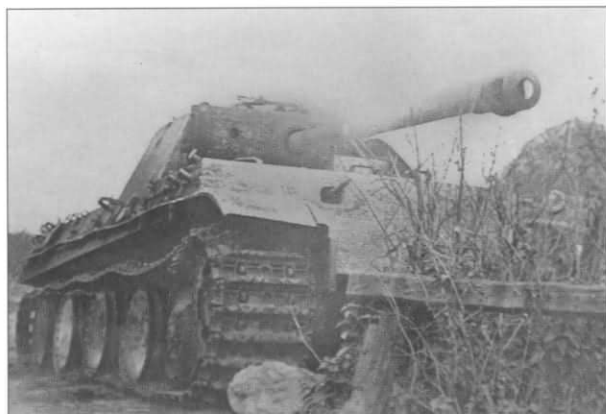
Two Pz.Kpfw.V Panther Ausf.G of 19.Panzer-Division, knocked out by Polish or Soviet forces in the Studzianki area. A fire has ravaged the first vehicle, burning off the rubber tires on the roadwheels. The fire weakened torsion bar suspension has collapsed lowering it noticeably to the ground. The other vehicle also appears to have some fire damage as well. The chassis number, '120734', can still be seen painted in black on the glacis, indicating that it was built in July 1944 at the M.A.N. assembly plant. 19.Panzer-Division was transferred back to Germany from the Eastern Front in May 1944 and was refitted as a 'Panzer-Division 44' in Holland in July/August 1944, with one battalion of Pz.Kpfw.V and one of Pz.Kpfw.IV. They were immediately sent back into action in Poland.
