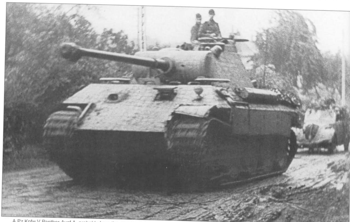
A Pz.Kpfw.V Panther Ausf.A, probably from the same unit, followed close behind by a staff car. The pattern in the zimmerit coating can be plainly seen and it appears that no camouflage paint or markings applied.
