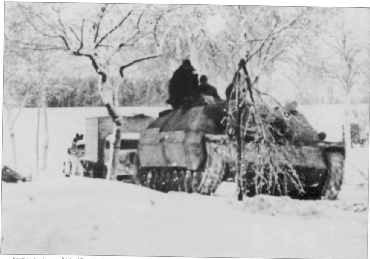
Another Jagdpanzer IV Ausf. F on the Western Front in the winter of 1944-45. The German firm Vomag produced 769 of these vehicles from January to November 1944. In August 1944, they began installing the longer barreled gun, the 7.5cm PaK42 L/70, in some vehicles. The new version was designated Panzer IV/70(V) which had completely replaced the Jagdpanzer IV by December 1944. The schürzen have been modified slightly by the crew of this vehicle. It appears that the brackets have probably been damaged and removed, allowing the schürzen to be bolted directly to the bracket mounting lugs welded to the superstructure. The schürzen were then bent down at that point.
