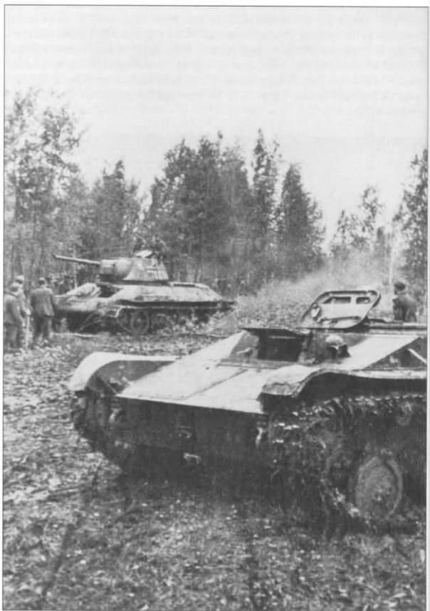
The Germans made extensive use of captured enemy equipment on all fronts during the war. The vehicle in the foreground is a Soviet T-60 light tank that has had its turret removed and is being used as an artillery tractor. In the background is a T34/76 Model 1943 which has a large white outline Balkenkreuz painted on the side of the turret along with a white outline Roman numeral 'II' in front of it. For obvious reasons, they were generally relegated to anti-partisan duties in rear areas.
