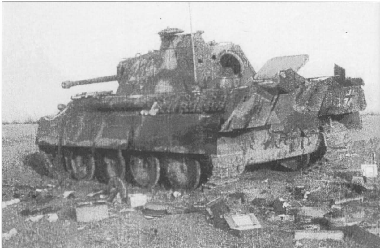
A late Pz.Kpfw.V Panther Ausf.G abandoned on a battlefield on the Eastern Front. The raised fan cover for the crew compartment heater, that was introduced in October 1944, can be seen on the engine deck although the vehicle is still fitted with the shielded exhaust pipes and not the 'flammvernichter' exhaust also introduced around the same time. The tactical number '239' is painted on the side of the turret in large red numbers with a white outline. Note the two penetrations in the 45mm thick rear plate of the turret.
