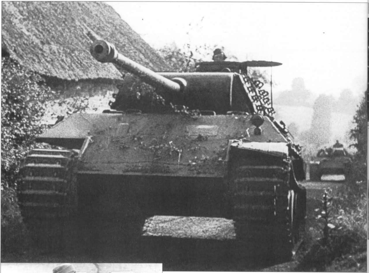
An old Pz.Kpfw.V Panther Ausf.D still in service on the Eastern Front in the late spring of 1944. The last of the Ausf.D production were built in August 1943 at which time the new Ausf.A made its appearance. The first Ausf.A, while fitted with the new commander's cupola, still retained the MG flap on the glacis.
