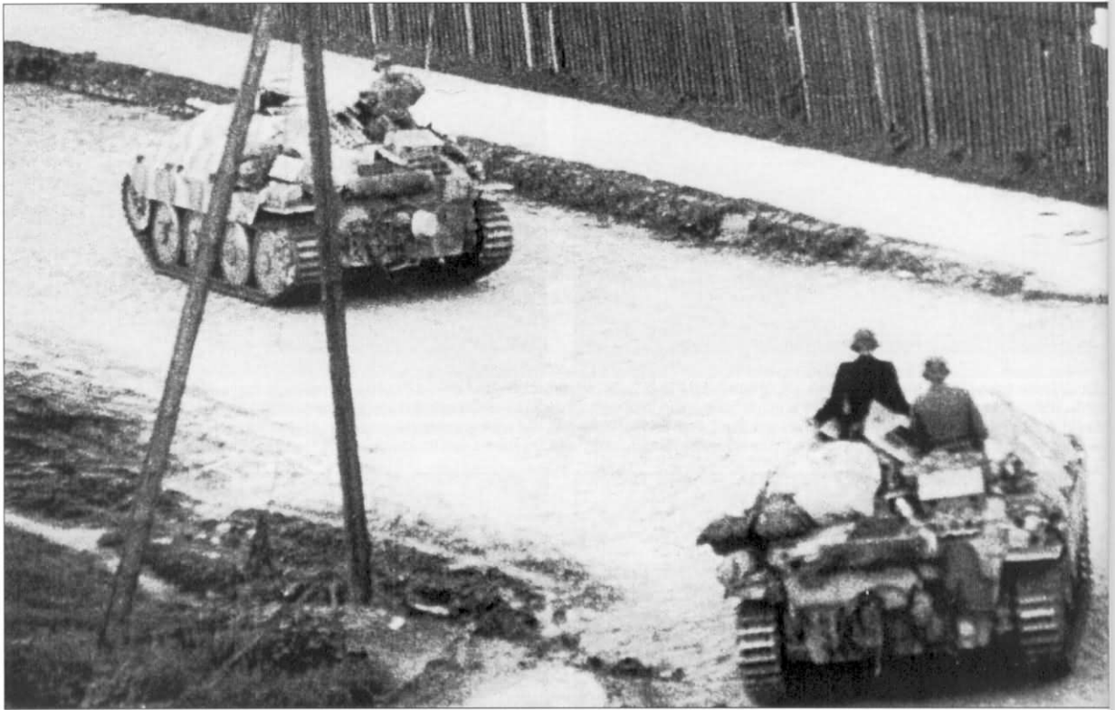
A pair of Jagdpanzer 38(t) 'Hetzer' tank destroyers used by the Germans against the Polish underground army in Warsaw at the beginning of August 1944. Production of these vehicles started in April 1944 and by July 1944, the first combat units began to receive them. They are painted in dark sand with a two color camouflage scheme of green patches with a dark brown outline, best seen on the lead vehicle in the background.
