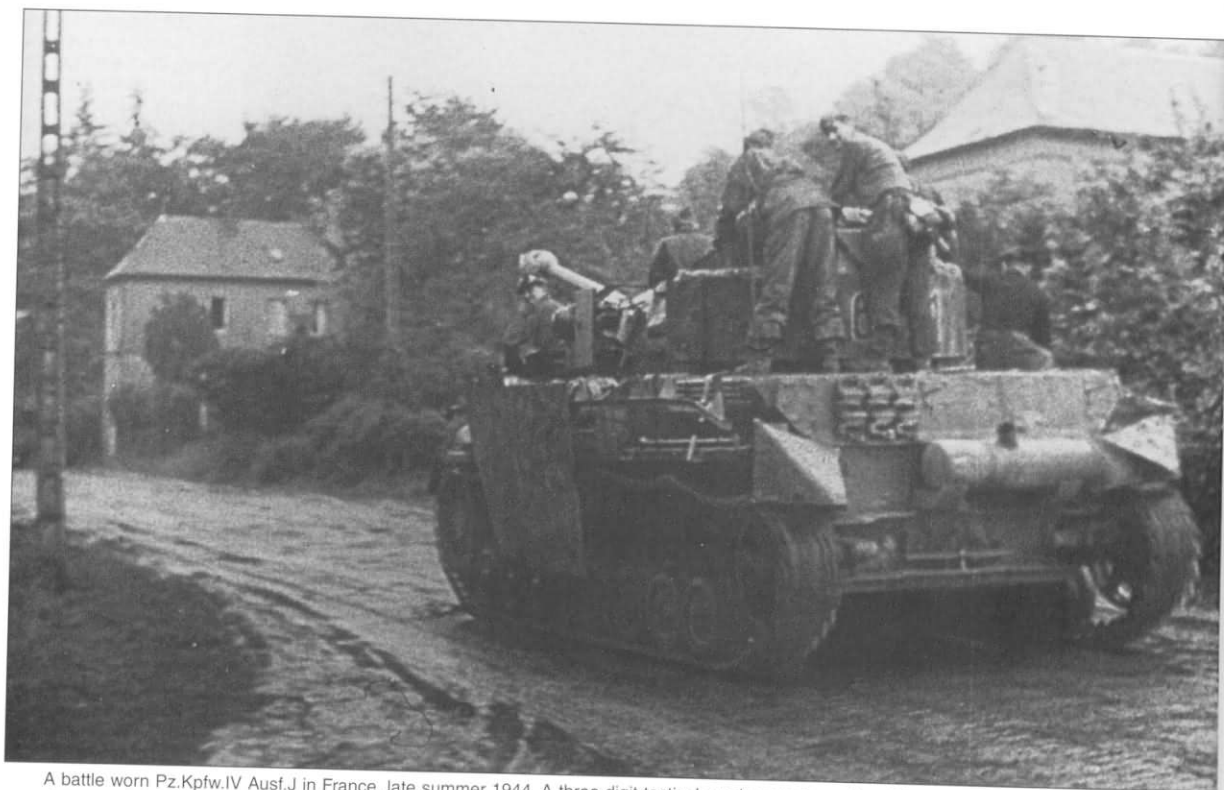
A battle worn Pz.Kpfw.IV Ausf.J in France, late summer 1944. A three digit tactical number starting with a '6' and ending with a '4' can be seen on the rear of the turret schürzen and is probably red with a white outline. The turret traverse motor was dropped in February 1944 and along with it, the small muffler that was mounted to the left of the main exhaust muffler.
