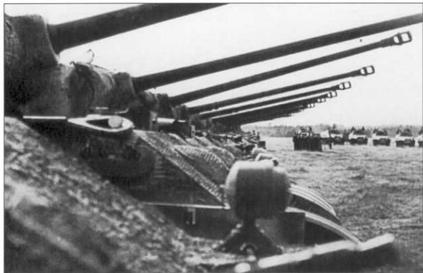
Twenty-two new Pz.Kpfw.V Panther Ausf.G lined up in a field somewhere in Germany, early autumn 1944. These were probably among the last Panthers built with zimmerit coating which was ordered to be dropped on September 9, 1944. In the background can be seen several Sd.Kfz.251/9 Ausf.D half-tracks armed with the 7.5cm KwK37 L/24 gun.
