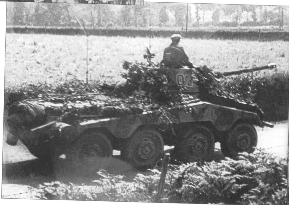
Command version of the Sd.Kfz.234/2 Puma equipped with additional radios and a star antenna mounted on the engine deck, most likely in France during the summer of 1944. The vehicle is painted in a three color camouflage scheme of green and brown over the dark sand base and has heavy foliage cover as well. On the turret, a tactical number, '023' or '025', is painted in black with a white outline. Of special interest is the very light color of the muzzle brake on the 5cm main armament.
