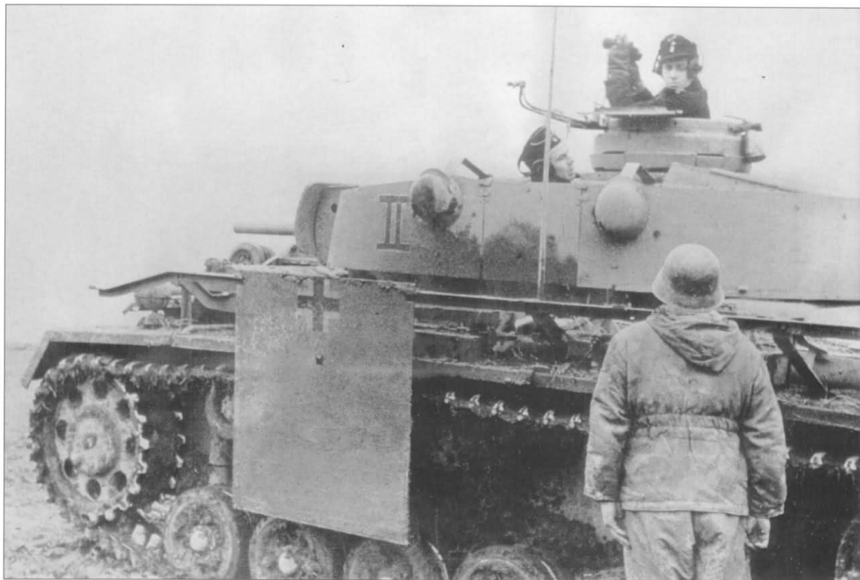
The commander of a Pz.Bef.Wg.III Ausf.J receives a communication from a courier in late 1943. 81 vehicles were produced from August to November 1942 with another 104 converted from Pz.Kpfw.III from March to September 1943. This one has been fitted with the early 8 hole drive sprockets with a spacer ring to accommodate the 40cm track. Not visible in the photo is the armored pot mount on the rear of the engine deck for the star antenna. It is finished in a scruffy coat of winter whitewash paint and, unusually, is equipped with the anti-aircraft mount for the MG34. The Roman numeral 'II', painted in black with a white outline, signifies a second battalion staff vehicle.
