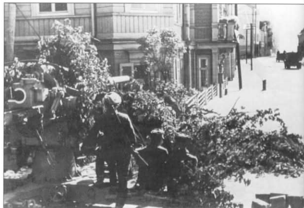
An 8.8cm FlaK 18 or 36 set up on a street in a Dutch city, September 1944. The camouflage and position of the gun suggest that they are prepared for a ground assault. The tall buildings would hinder its use in an anti-aircraft role.
