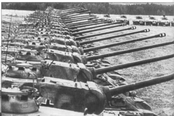
Twenty-two new Pz.Kpfw.V Panther Ausf.G lined up in a field somewhere in Germany, early autumn 1944. These were probably among the last Panthers built with zimmerit coating which was ordered to be dropped on September 9, 1944. In the background can be seen several Sd.Kfz.251/9 Ausf.D half-tracks armed with the 7.5cm KwK37 L/24 gun.
