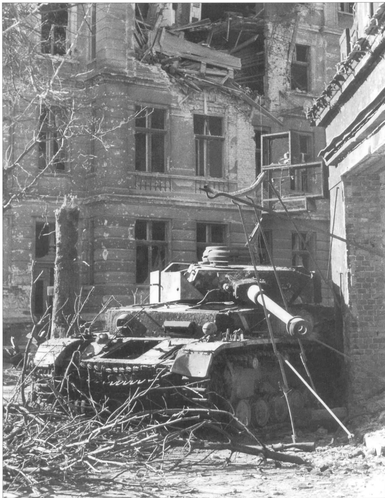
The wreckage of a Pz.Kpfw.IV Ausf.H in Kolberg in the spring of 1945. An internal explosion has blown off the transmission cover plate and driver's hatch and fire consumed the rubber from the roadwheels and return rollers. Note the unusual zimmerit pattern on the front plate of the superstructure.
