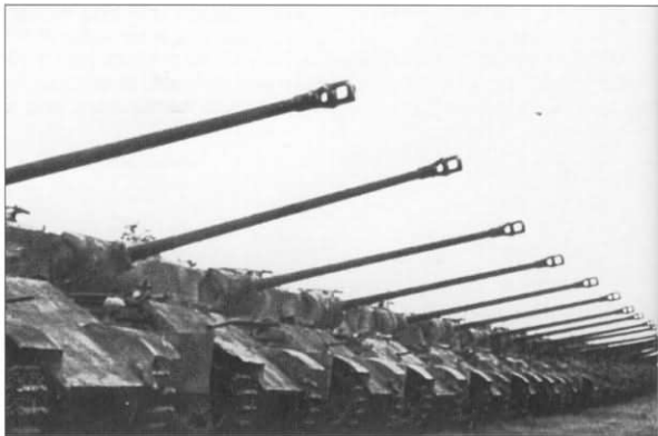
Twenty-two new Pz.Kpfw.V Panther Ausf.G lined up in a field somewhere in Germany, early autumn 1944. These were probably among the last Panthers built with zimmerit coating which was ordered to be dropped on September 9, 1944. In the background can be seen several Sd.Kfz.251/9 Ausf.D half-tracks armed with the 7.5cm KwK37 L/24 gun.
