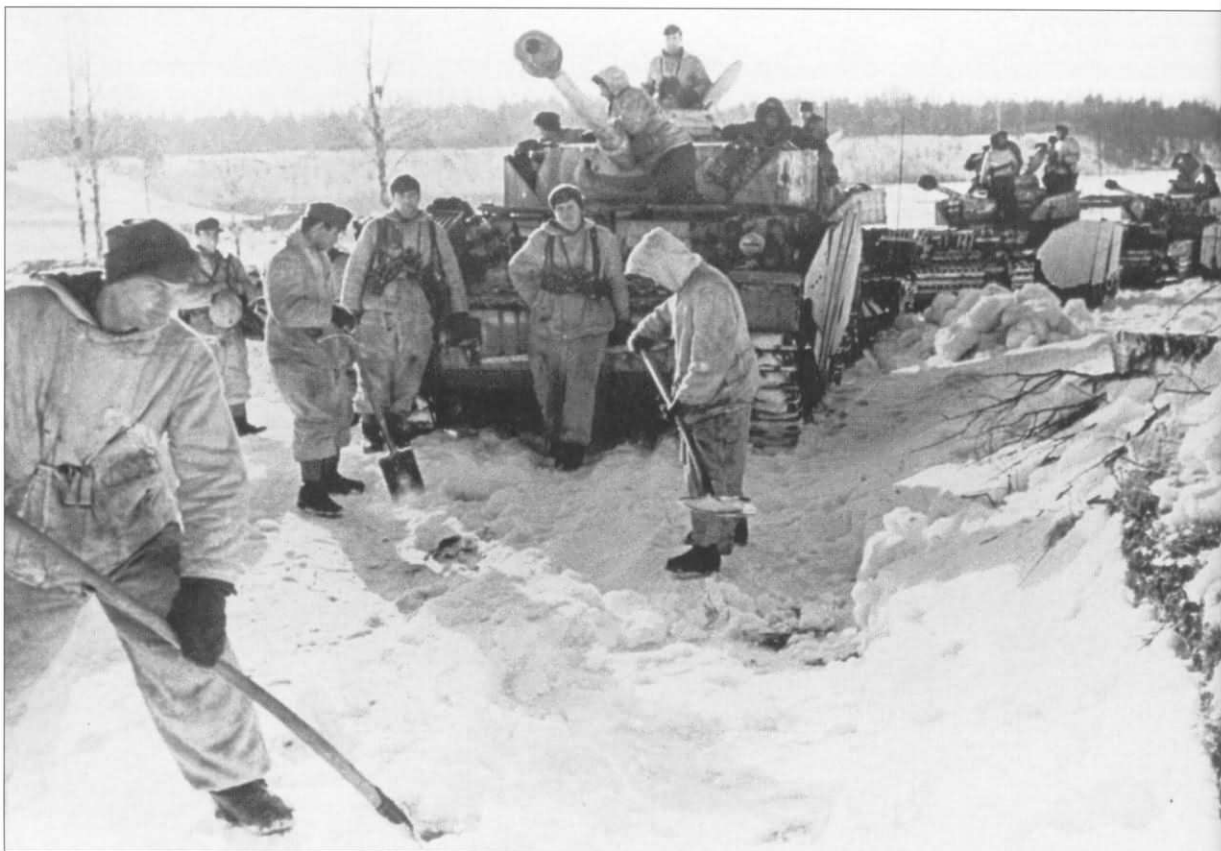
German infantry help clear a path through the deep snow to provide passage for a column of Pz.Kpfw.IV Ausf.H from an unidentified Panzer-Division in March 1944. Deep snow had the same effect as mud on an armored vehicle. If the vehicle bottomed out, the tracks would spin freely immobilizing it. On the leading tank, a Balkenkreuz with a white outline can be seen on the turret schürzen followed by a tactical number beginning with a '2'.
