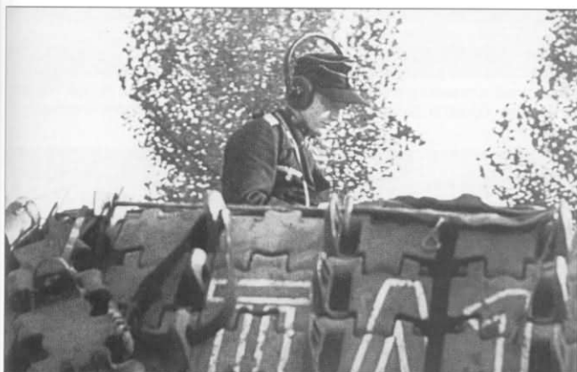
Two photographs of a Pz.Bef.Wg.V Panther Ausf.G from an Army Panzer-Division. It has several rows of spare track links hanging from the side of the turret to bolster its armor protection which was common during the later stages of the war. The white outline tactical number 'IIA1' indicate it is a staff vehicle in second battalion.
