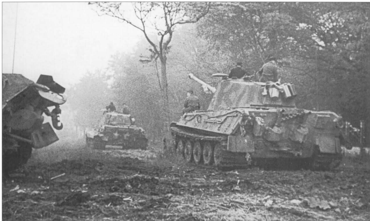
Three Pz.Kpfw. Tiger Ausf.B from s.Pz.Abt.503 after their arrival in Hungary in October 1944. The one on the right is an older vehicle and does not have the spare track hangers on the turret introduced in June 1944. Part of the tactical number '2?0', painted in red with a white outline, can be seen under the pail hanging over the rear turret hatch.
