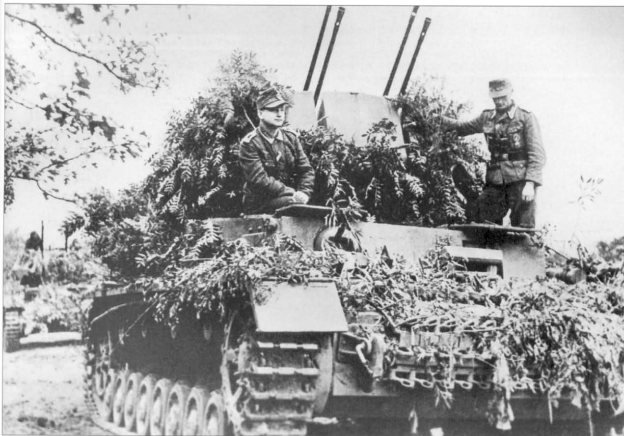
Another new vehicle to the Panzerwaffe in 1944 was the Flakpanzerkampfwagen IV (2cm Flakvierling 38) (Sd.Kfz.161/4) self-propelled anti-aircraft gun, known as the 'Wirbelwind'. These were assembled on rebuilt Pz.Kpfw.IV chassis that had been returned to Germany. This one is based on a Pz.Kpfw.IV Ausf.G identifiable by the 30mm armor plates welded to the front of the hull and superstructure. The first 17 were completed in July 1944 and, starting in September, began to be issued to the various units on the basis of four 'Wirbelwind' and four 'Möbelwagen' each.
