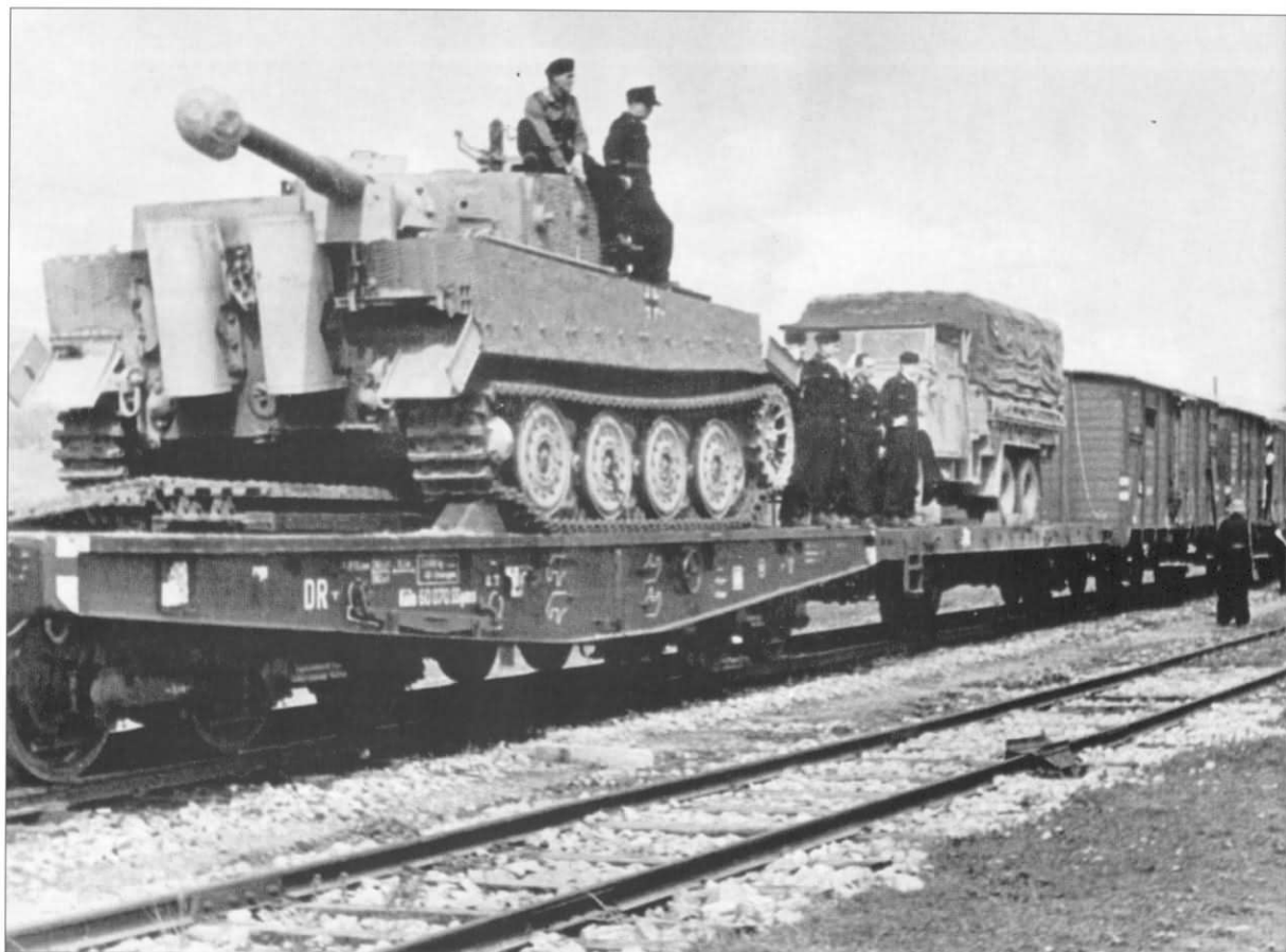
A new Tiger I sits on a railway flatcar on its way to Panzer-Division 'Großdeutschland' in May 1944. There are no visible markings but the distinctive cuffband of the division can be seen on some of the crew uniforms. The vehicle has been prepared for rail transport following standard procedures with the narrow transport tracks installed, the side mudguards removed and the turret traversed to the rear with the gun barrel securely blocked with a wooden cradle. The wide battle tracks can be seen stowed underneath the vehicle.
