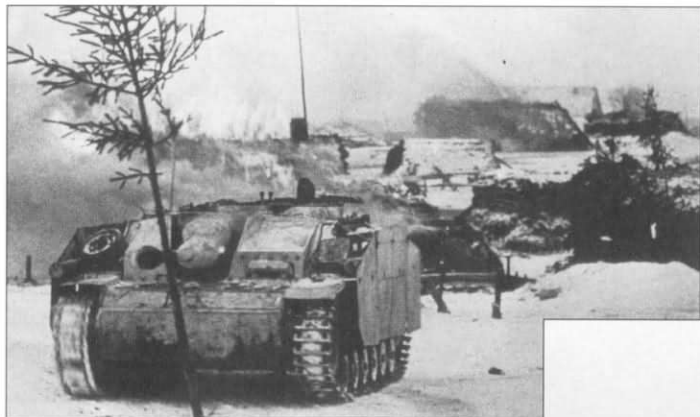
A late StuG.III Ausf.G advances through a burning village near Vitebsk in March 1944. It is fitted with the 'topfblende' cast gun mantlet and shot deflector in front of the cupola that were installed on Sturmgeschütz produced starting in the fall of 1943. Since the spring of 1943, Sturmgeschütz were used to create a new III.Abteilung in some of the Panzer-Divisions to increase their operational strength due to low production rates for the more expensive standard gun tanks.
