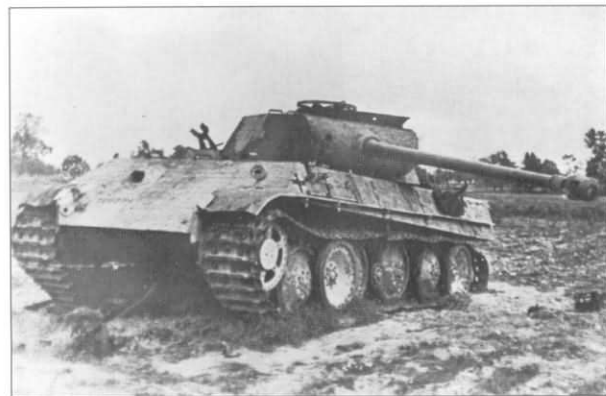
Two Pz.Kpfw.V Panther Ausf.G of 19.Panzer-Division, knocked out by Polish or Soviet forces in the Studzianki area. A fire has ravaged the first vehicle, burning off the rubber tires on the roadwheels. The fire weakened torsion bar suspension has collapsed lowering it noticeably to the ground. The other vehicle also appears to have some fire damage as well. The chassis number, '120734', can still be seen painted in black on the glacis, indicating that it was built in July 1944 at the M.A.N. assembly plant. 19.Panzer-Division was transferred back to Germany from the Eastern Front in May 1944 and was refitted as a 'Panzer-Division 44' in Holland in July/August 1944, with one battalion of Pz.Kpfw.V and one of Pz.Kpfw.IV. They were immediately sent back into action in Poland.
