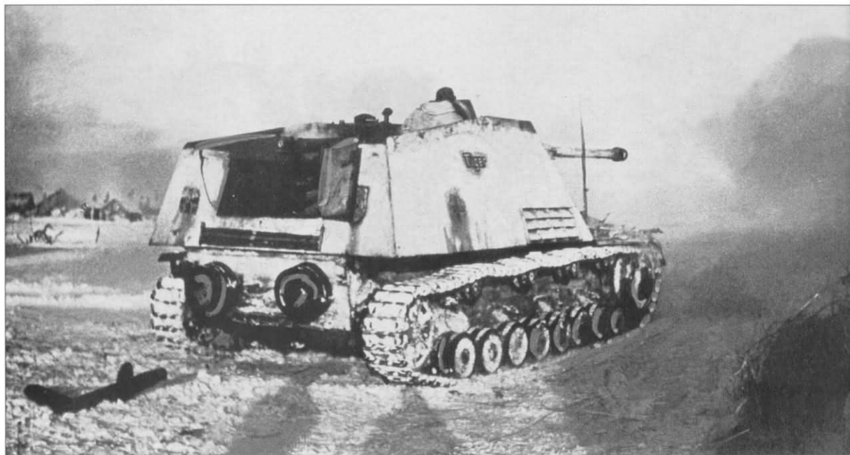
A 'Nashorn' self-propelled anti-tank gun, mounting the deadly 8.8cm PaK43/1 L/71, fires at an enemy target during one of the Eastern Front battles in the winter of 1943-44. In addition to its white winter camouflage paint, the vehicle carries the name 'Tiger' on the side along with a white outlined Balkenkreuz, also repeated on the left rear. A large unit emblem in the shape of a shield can be seen just behind the open right rear access door but, unfortunately, is not clear enough to be identified. The 'Nashorn' was introduced in time for the battle at Kursk in July 1943 and proved to be a highly effective tank killer unit in the East. It was replaced in 1944 by the Jagdpanzer IV and Jagdpanther.
