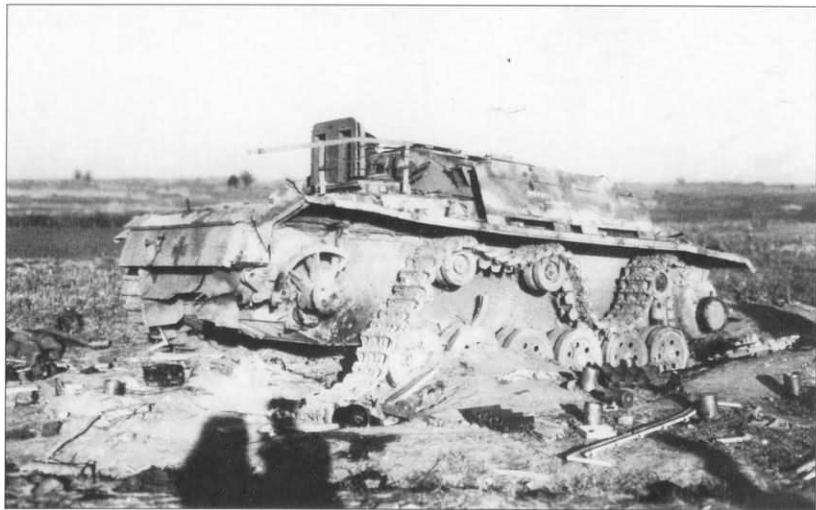
A StuH 42 Ausf.G also destroyed in the same raid. This was a later model vehicle that was prepared for, but not fitted with, the remote control MG mount, but still fitted with side opening loader's hatches. These vehicles may be from a much photographed, but as yet unidentified, Sturmgeschütz-Abteilung that field modified the schürzen plates to hang from short pieces of pipe welded to angles attached to the mudguards. The modified brackets can be clearly seen. Note the 10.5cm casings littering the ground around the vehicle.
