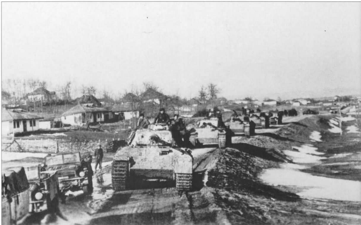
A column of Pz.Kpfw.V Panther Ausf.A from Panzer-Regiment 'Großdeutschland' and other divisional soft-skin vehicles on a road near Jassy, Romania in early April 1944. Most of the snow has disappeared but the ground is still firmly frozen as can be seen by the condition of the dirt road these vehicles are traveling on. These are early production Ausf.A fitted with the new cast cupola but still retaining the MG flap in the glacis.
