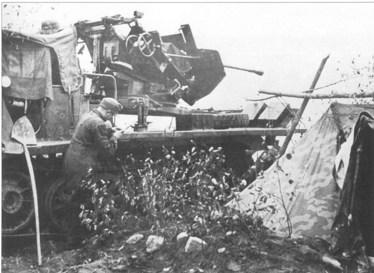
An Sd.Kfz.7/2 self-propelled anti-aircraft gun on station in October 1943. The mounting of the 3.7cm FlaK36 anti-aircraft gun is clearly shown. Judging from the tent made up of Army splinter pattern Zeltbahn shelter quarters, it is possibly attached to a Wehrmacht Heer unit, although Luftwaffe troops were also issued with the Zeltbahn as well.
