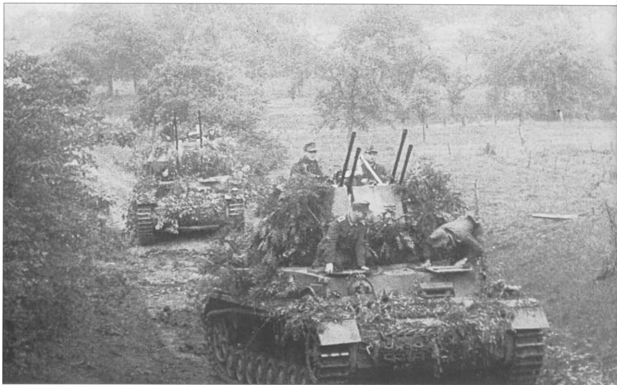
Two Flakpanzer IV 'Wirbelwind' photographed in early October somewhere on the Western Front. They have also been built on Pz.Kpfw.IV Ausf.G chassis and have standard three color camouflage paint schemes consisting of green and brown patches on the dark sand base. As usual, they have been liberally covered with branches to improve their camouflage. A total of 122 vehicles were completed by the end of March 1945.
