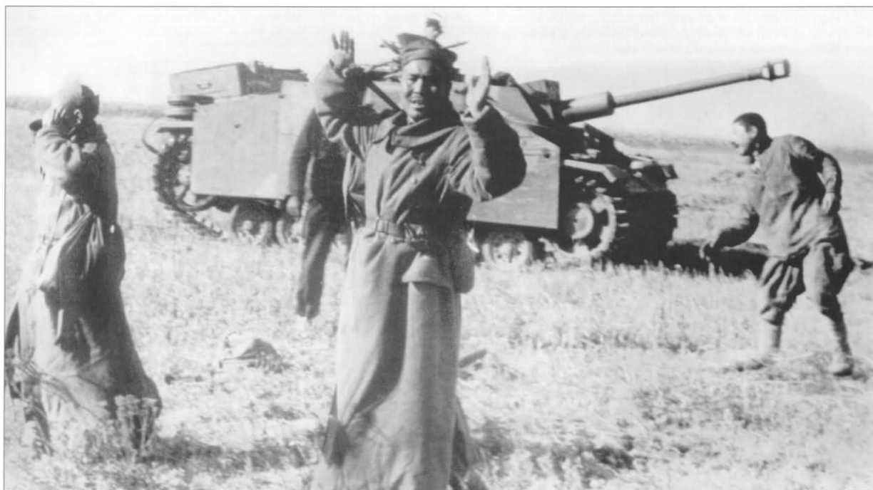
Surrendering Soviet troops are taken into captivity by German infantry supported by a StuG.III Ausf.G. It could be from one of the independent Sturmgeschütz Abteilungen or possibly one of the Panzer-Divisions which started to be equipped with these vehicles in their newly created III.Abteilung starting in April 1943. A camouflage scheme of large brown patches has been sprayed over the dark sand base which was common for the early spring and autumn seasons.
