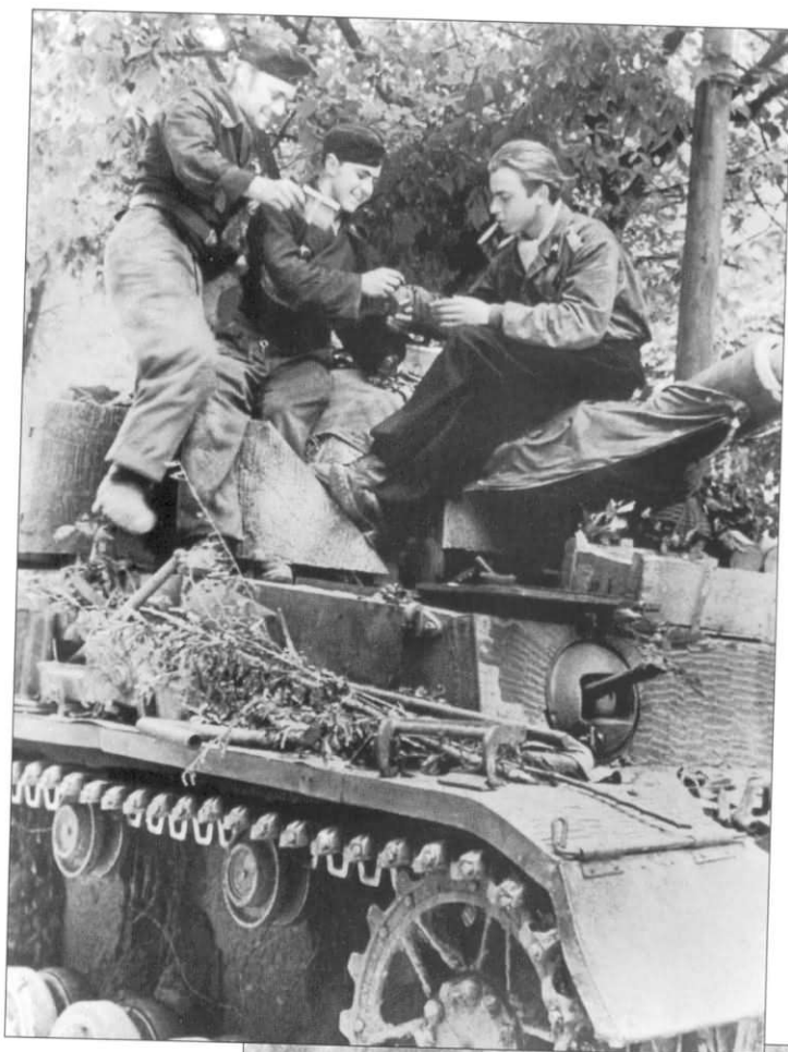
The crew of this Pz.Kpfw.IV Ausf.H enjoy a cigarette break in France during the summer of 1944. The vehicle is fitted with the newer drive sprocket and all steel return rollers which were introduced in the previous year along with a single 80mm front plate and zimmerit anti-magnetic mine coating.
